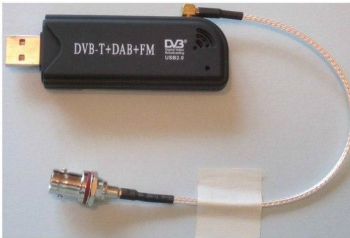
FIGURE 3. RTL tuner (with R820T and Realtek RTL2832U inside) and BNC adapter cable.
